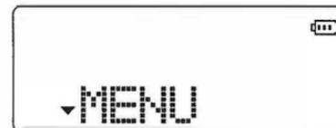
**Note:** Under channel mode, the following menu settings are invalid: CTCSS,DCS,W/N,PTT-ID,BCL,SCAN ADD TO,S-CODE,CHANNEL NAME. Only the H/L power could be changed by pressing '#'.
